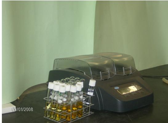
Figura 33 – Digestor HACH
