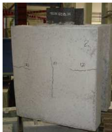
Ruptura da laje (Vianna, 2009)
