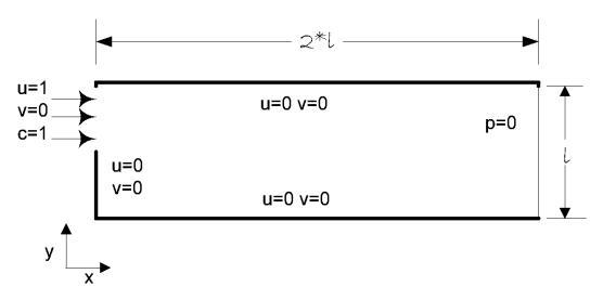
Figure 6.1: 2D Domain with Boundary Conditions.
