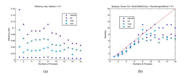
Figure 6.9: Efficiency Ratio and Speedup for Method 1 - Problem 1: (a) Efficiency Ratio. (b) Speedup.
