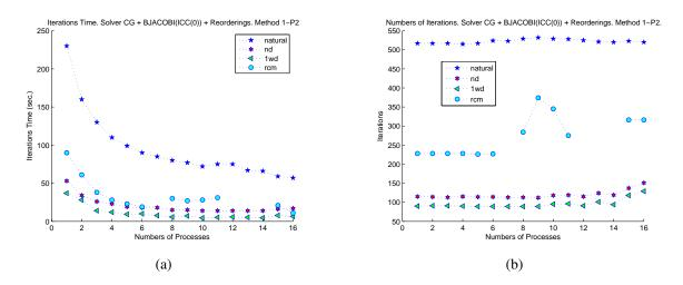
Figure 6.12: Number of Iterations and Time for Method 1. Problem 2: (a) Iterations Time in seconds. (b) Number of Iterations.
