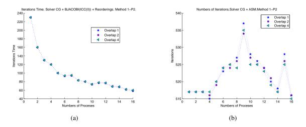
Figure 6.14: Time and Iterations Time for Solver CG with ASM preconditioner Method 1- Problem 2 : (a) Iterations Time in seconds. (b) Numbers of Iterations.
