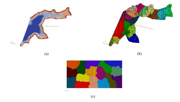
Figure 4.4: Examples of Mesh Partitioning for different domains: (a) Example of a Reservoir Branch. (b) Mesh of the Reservoir Branch after the decomposition. (b) Rectangular Domain Partitioned with 16 processes.
