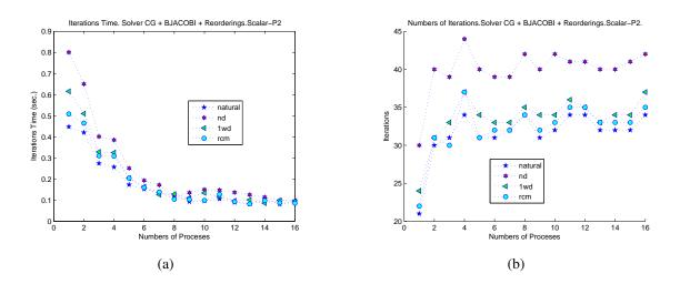
Figure 6.31: Execution Time and Iteration count for Scalar Concentrations in Problem 2: (a) Execution Time (sec.). (b) Iteration count.
