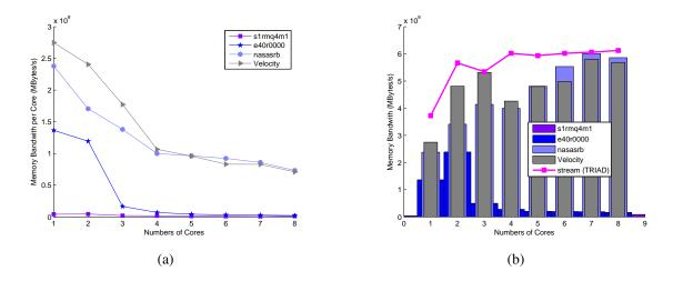
Figure 5.5: Memory Bandwidth Achieved for each matrix: (a) Memory Bandwidth Measured per Core. (b) Total Memory Bandwidth Measured with core increase.
