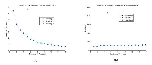
Figure 6.22: Number of Iterations and time. Method 2 - Problem 2: (a) Time in seconds. (b) Iterations.
