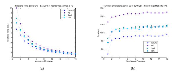
Figure 6.20: Number of Iterations and Time for Method 2. Problem 2: (a) Iterations Time in seconds. (b) Number of Iterations.
