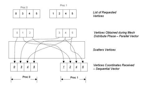
Figure 4.5: Sketch of the scatters vertices algorithm.
