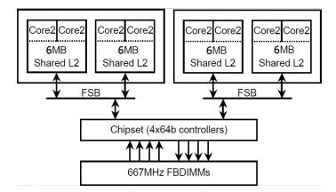
Figure 5.2: Architectural overview for dual-socket×quad-core Intel Harpertown.
