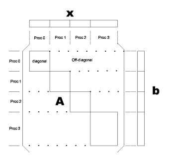
Figure 3.4: Matrix Parallel Layout used on PETSc.
