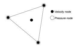
Figure 2.2: 2D Mini Element.
