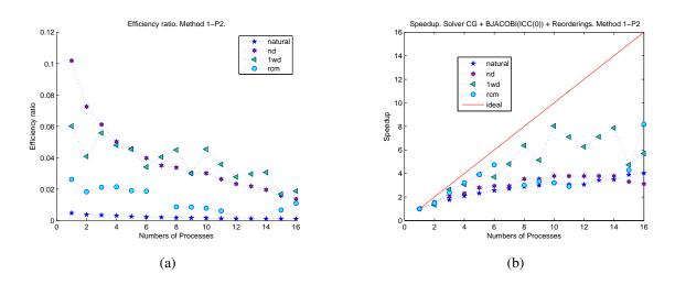
Figure 6.13: Efficiency Ratio and Speedup for Method 1 - Problem 2: (a) Efficiency Ratio. (b) Speedup.
