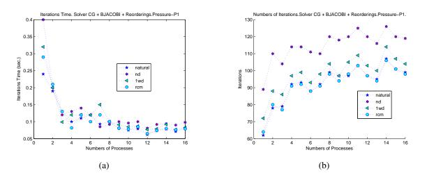
Figure 6.25: Execution Time and Iteration count for Pressure in Problem 1: (a) Execution Time (sec.). (b) Iteration count.
