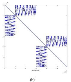
Figure 2.3: Typical Sparsity Pattern for our problem: (a) Sparsity Pattern for Matrix K . (b) Sparsity Pattern for Matrix M.
