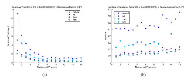
Figure 6.8: Number of Iterations and Time for Method 1. Problem 1: (a) Iterations Time in seconds. (b) Number of Iterations.
