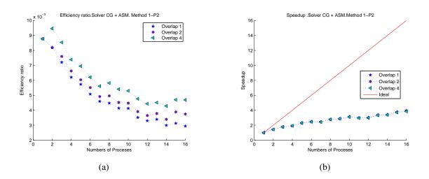
Figure 6.15: Speedup and efficiency for CG+ASM. Method 1-Problem 2: (a) Efficiency Ratio. (b) Speedup.
