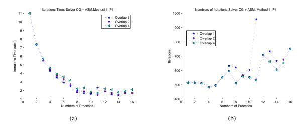
Figure 6.10: Time and Iterations Time for Solver CG with ASM preconditioner Method 1- Problem 1 : (a) Iterations Time in seconds. (b) Numbers of Iterations.
