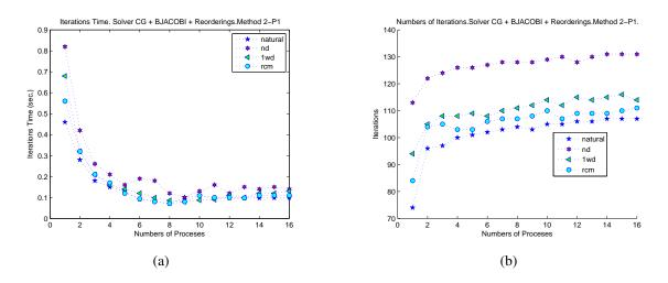
Figure 6.16: Number of Iterations and Time for Method 2. Problem 1: (a) Iterations Time in seconds. (b) Number of Iterations.
