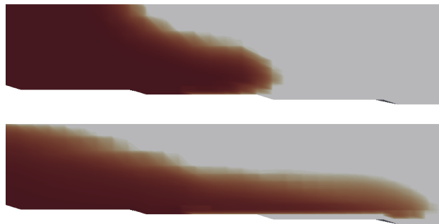
Figure 6.6: Numerical simulation of gravity current wave propagating along the tributary.
