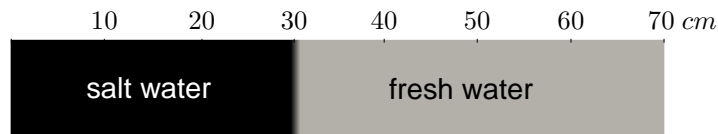
Figure 6.1: Initial configuration of the 2D gravity current simulation.
