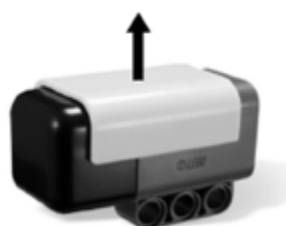
Figura 11 – NXT Gyro Sensor, da HiTechnic Products .
