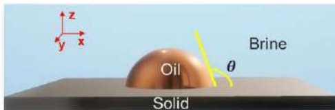
Fig. 1. Sketch of the oil droplet immersed in brine resting on a flat solid particle.
