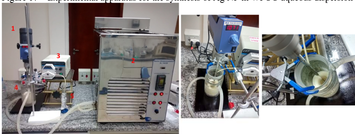
Figure 17 – Experimental apparatus for the synthesis of Ag NP in WPUU aqueous dispersion
