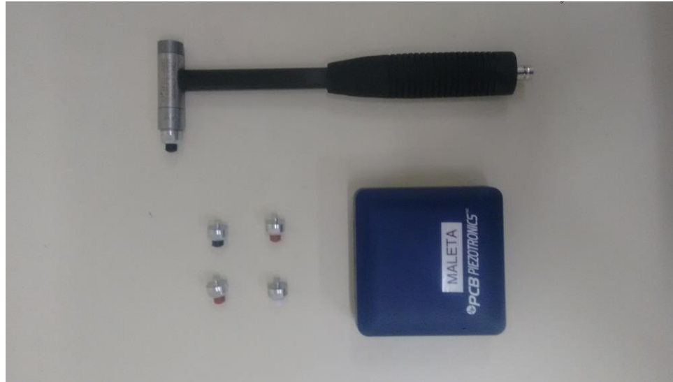
Figura 51 – Martelo ICP® IMPACT HAMMER 086C03 PCB Piezotronics
