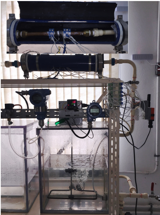
Fig. 3. The measuring system prototype and close view of the thermal flow meter.
