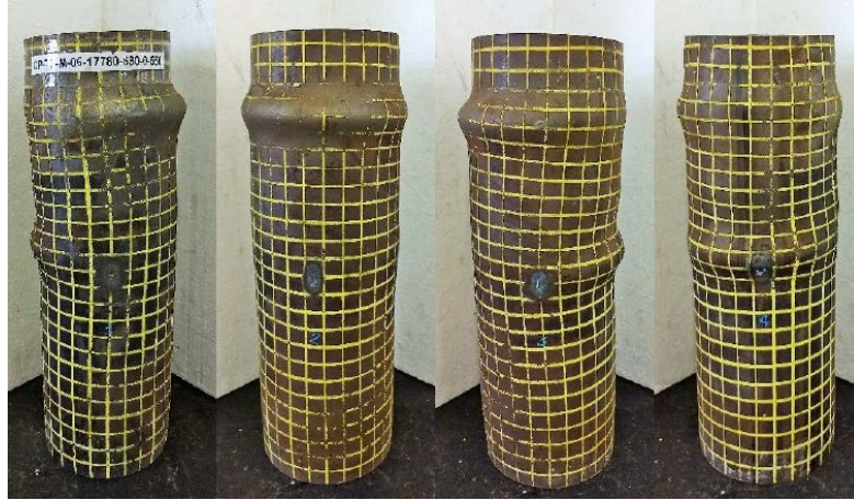
Figure 43 - Typical failure modes of CFST columns with RAC [39].
