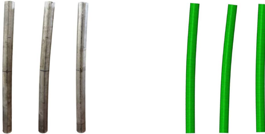
Figure 15 - Experimental and numerical deformations of columns with CHS 89 x 3, 1200 of length and RCA replacement ratio of 0%, 35% and 70% [40].
