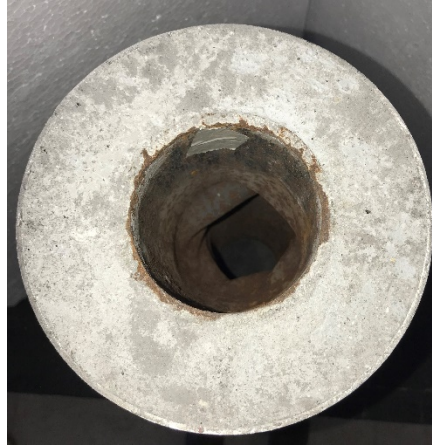
Figure 40 - Specimen RAC1 after testing showing an inward-only local buckling of the carbon steel inner tube.
