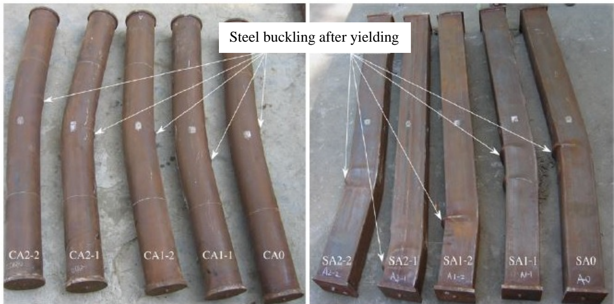
Figure 12 - Failure mode of the RAC CFST columns [30].
