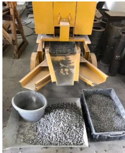
Figure 33 - View of the crushed concrete to make the RCA.
