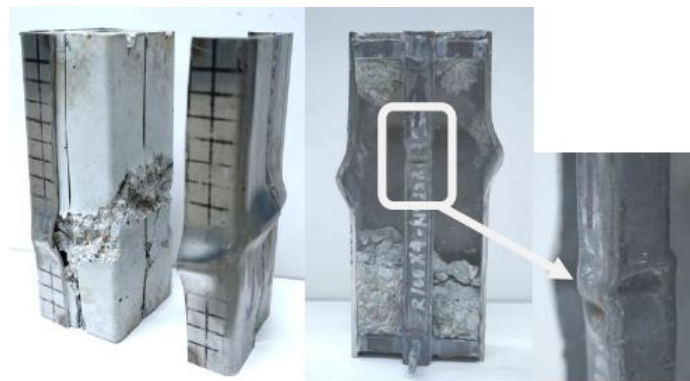
Figure 24 - CFDST columns failure modes [9].
