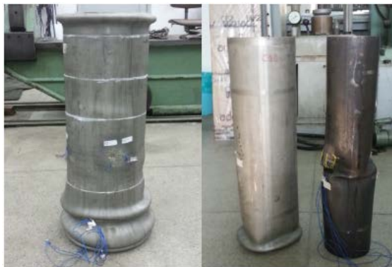
Figure 25 - Failure modes of the CFDST columns [47].
