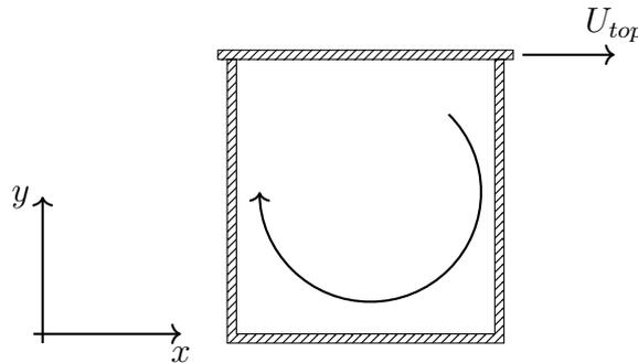
The benchmark problem were simulated with the following Reynolds numbers ( $Re$ ): 10, 100, 400 and 1000. The Figure 23 and Figure 24 present the profile of the horizontal and vertical velocities, respectively, for steady state in several Reynolds number. They were compared with Ghia et al. (1982) [11] and Marchi et al. (2009) [12]. The domain was discretized using a linear triangular mesh with 1563 nodes and 2988 elements.
