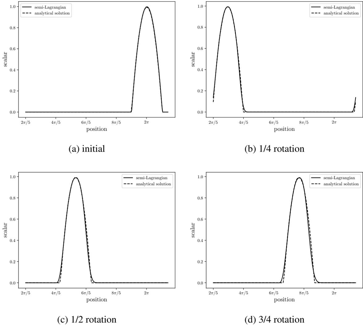
The Figure 28 and Figure 29 show the spatial and temporal evolution of the scalar profile for the semi-Lagrangian Method in an unstructured linear and quadratic triangular mesh respectively. As mentioned earlier, the spurious oscillations are not presented in both simulations. However, in the Figure 28, it is possible to observe the numerical diffusion, making its use not recommended for high Reynolds number problem.
