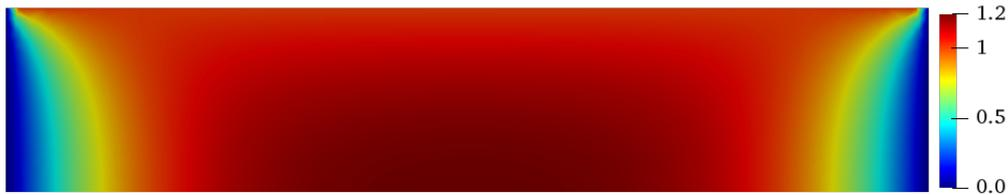
Figure 7: Numerical solution of the heat equation for a triangular mesh with 1357 nodes and 2712 elements. The color represents the temperature with blue being the lowest value and red the highest.
