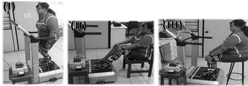
Fig. 1. A volunteer performing WBVE in the squatting posture ( posture I ), sitting with ankle at free angulation ( posture II ), and with ankles perpendicular to VP ( posture III ), with the digital accelerometers and goniometers positioned.
