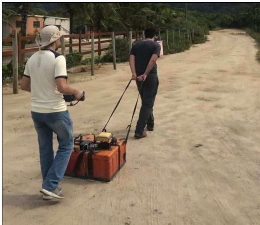
Figura 5 – Levantamento de Ground Penetrating Radar (GPR).
