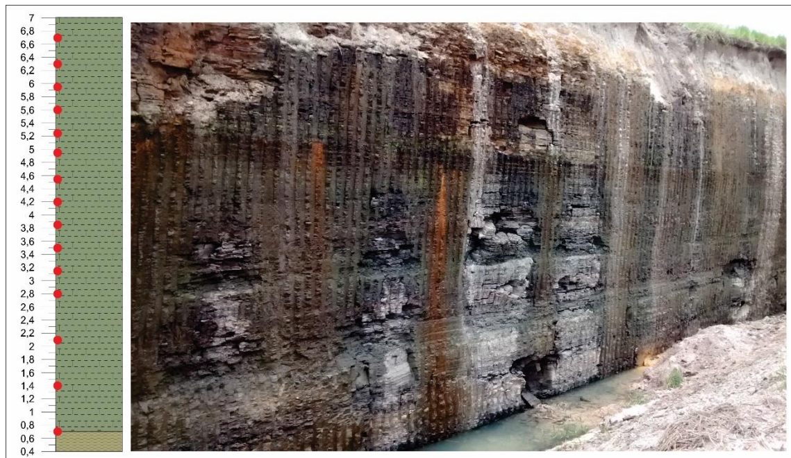
Figure 3 - Schematic profile with red sampling points at Fazenda Extrativa Santa Fé- Ltda in Tremembé, São Paulo State
