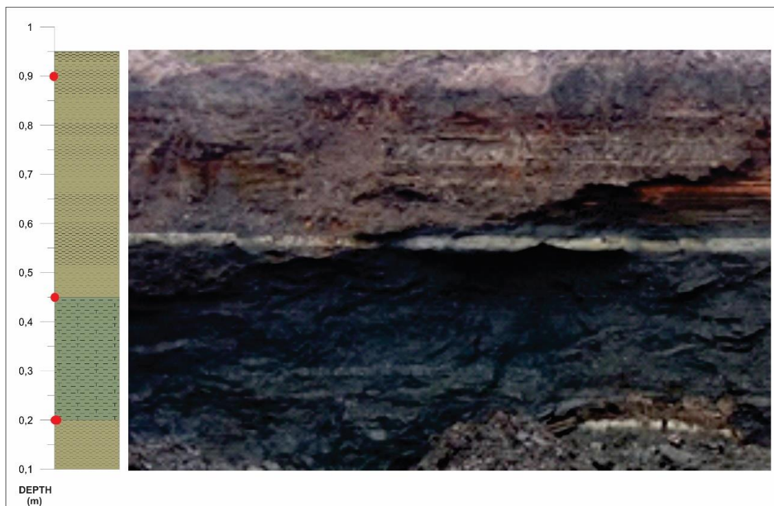
Figure 4 - Schematic profile with red sampling points at Aligra – Indústria e Comércio de Argila Ltda, in Tremembé, São Paulo State.
