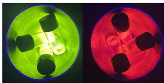
Fig. 1. \text{Eu}^{3+} and \text{Tb}^{3+} -ketoprofen complexes and their respective luminescence, when irradiated with a U.V lamp (28 W, \lambda = 365 nm).
