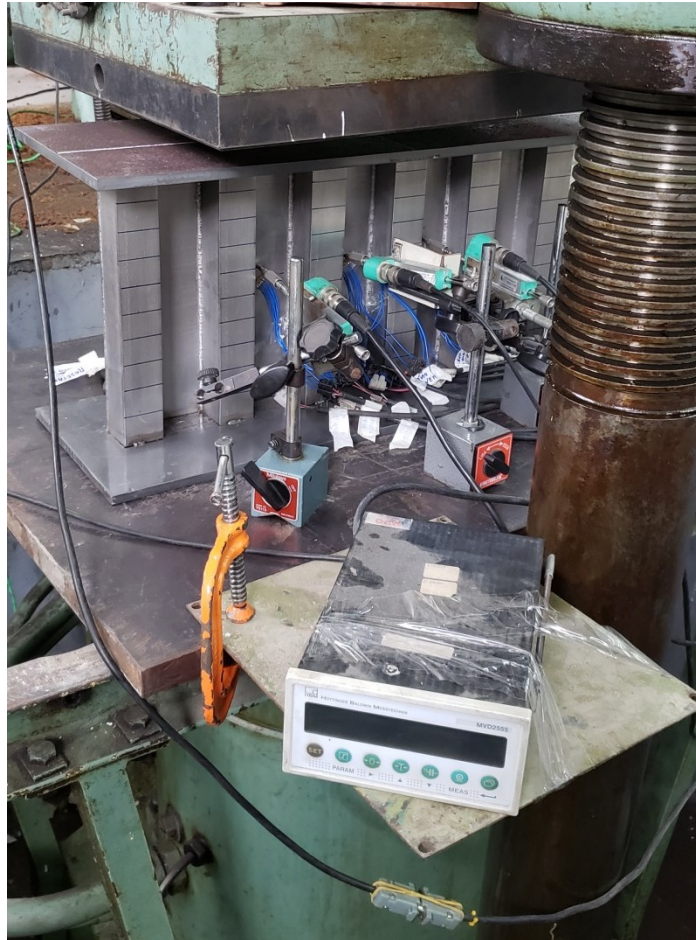
Figura 63 – LVDTs e strain gauges – Vista frontal - Painei 2
