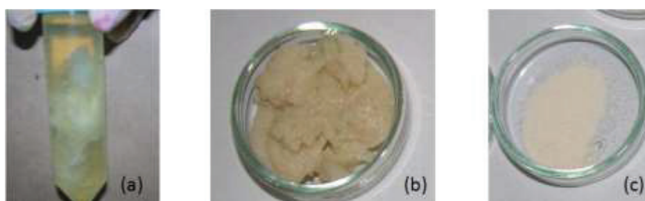
Fig. 1. the aspect of xanthan gum after: (a) Precipitation with ethanol; (b) Spinning; (c) drying and grinding.
